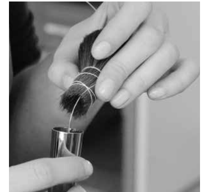
4. Einbringen in die Zwingen Filling the ferrule with the hair bundle
